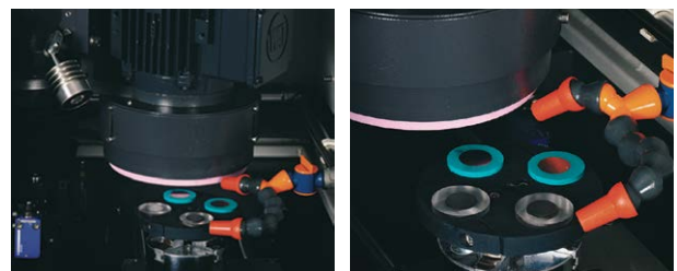
Ergonomic operation resulting in high quality planar surface, thus saving time on the next preparation steps
