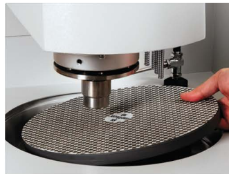
Simple exchange of working discs
