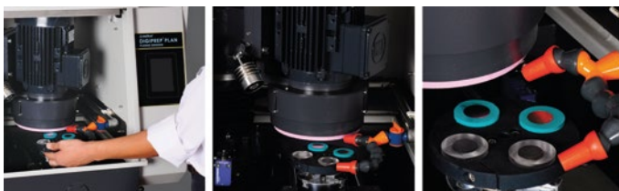
Ergonomic operation resulting in high quality planar surface, thus saving time on the next preparation steps
