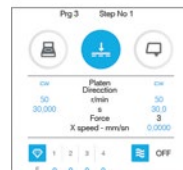
Programmable HMI touch screen controls
