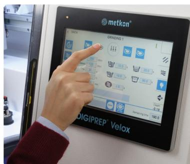
Programmable HMI touch screen controls
