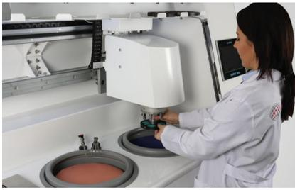
DIGIPREP Velox Fully Automatic Programmable Grinding/Polishing System is developed for operator free sample preparation for high volume sample throughput starting from planar/coarse grinding to cleaning and drying. You only need to place the sample holder, select the program number for your specific application and depress the “Start” button. That’s it! Your samples will be ready for analysis fully automatically.
