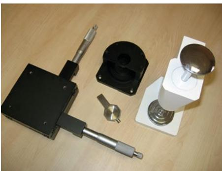
Several different optional accessories such as "Specimen Holders", "Indentors", "X-Y Stages" etc. are available for different applications.
