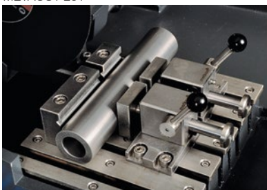
Stainless steel clamping devices and T-Slotted table
