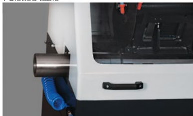
Side access port for extra-long workpieces
