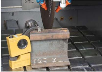
**SERVOCUT 602 is an advanced high capacity cutting machine especially designed for cutting extra-large and multiple specimens.**
