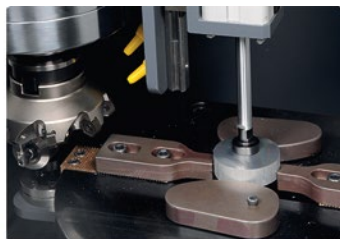
Automatic Clamping And Sample Height Measurement
